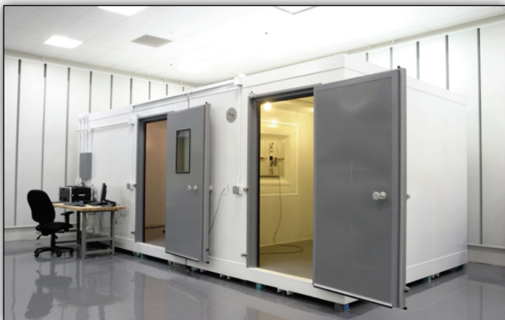
K&STLE KαBIN - Self Contained Acoustic Test Facility
